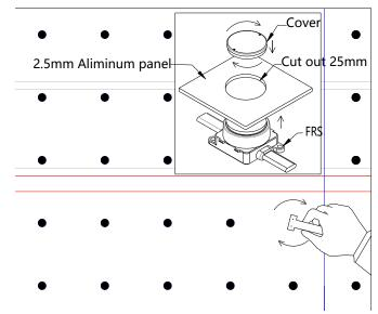
4 Use a special tool to tighten the cover on the front of the aluminum plate to secure the module.
