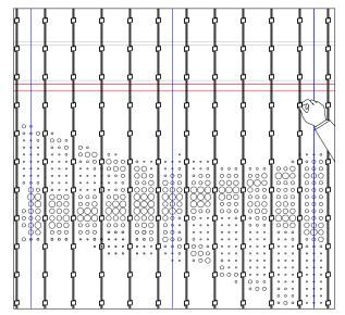
Place the modules on the back of the aluminum plate, ensuring that each module is aligned with the aluminum plate holes.
