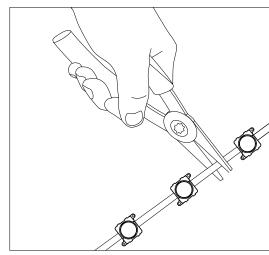
Measure and cut FRS LED strip to the appropriate length for each Aliminum panel. Cuts can be made between any of the modules.
