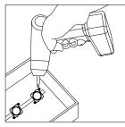
Use screws to secure at every FRVS LED module within the Light box. Use #6 (M3) pan headed metal screws.
