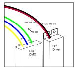
Run a wire from the Power Supply and DMX Decoder to each Light box and connect to the first LED module on the strip.
