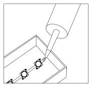
Must apply electrical grade silicone to exposed wires.
