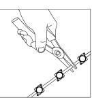
Measure and cut FRVS LED strip to the appropriate length for each Light box . Cuts can be made between any of the
