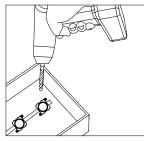
Drill a 10 mm hole near the FRVS LED strip and grommet the hole for supply wire access.
