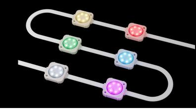
FRM Series is an extra bright dot with 6 LEDs per dot casing. The dots are constructed on a flexible cable with a customizable pitch. The dots are single dot controllable by DMX, and are connected per string using the Pixel Distributor. The Pixel Distributors can be daisy chained to form large installations
