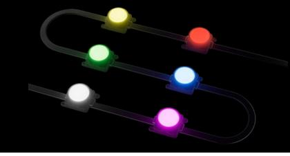
FRS Series is an extra bright dot with 6 LEDs per dot casing. The dots are constructed on a flexible cable with a customizable pitch. The dots are single dot controllable by DMX, and are connected per string using the Pixel Distributor. The Pixel Distributors can be daisy chained to form large installations
