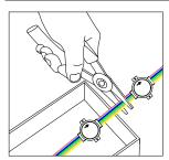
Measure and cut FRL LED strip to the appropriate length for each Light box. Cuts can be made between any of the modules.
