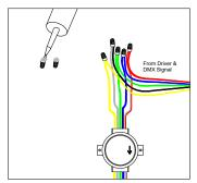
3 Connection follow wiring diagram instructions. Connect LED strips using twist-on wire connectors.
