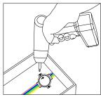
3 Use screws to secure at every FRL LED module within the Light box. Use #6 (M3) pan headed metal screws.
