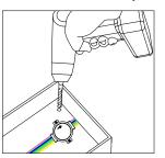
4 Drill a 10 mm hole near the FRL LED strip and grommet the hole for supply wire access.
