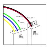
2 Run a wire from the Power Supply and DMX Decoder to each Light box and connect to the first LED module on the strip.
