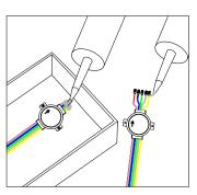
Must apply electrical grade silicone to exposed wires.
