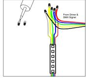
3 Connection follow wiring diagram instructions. Connect LED strips using twist-on wire connectors.
