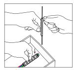
Remove tape backing and stick FLL LED modules into place. Continue until you have reached the end of the strip.
