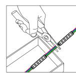
Measure and cut FLL LED strip to the appropriate length for each Light box. Cuts can be made between any of the modules.
