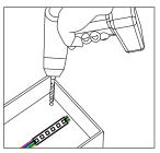
Drill a 10 mm hole near the FLL LED strip and grommet the hole for supply wire access.
