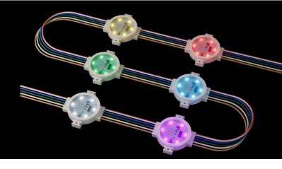
FRL Series is an extra bright dot with 6 LEDs per dot casing. The dots are constructed on a flexible cable with a customizable pitch. The dots are single dot controllable by DMX, and are connected per string using the Pixel Distributor. The Pixel Distributors can be daisy chained to form large installations
